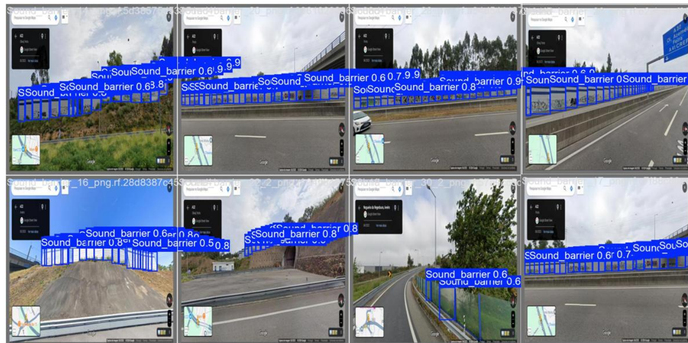
Fig.2: Prediction result on Sound Barriers identification using YOLOv10n
