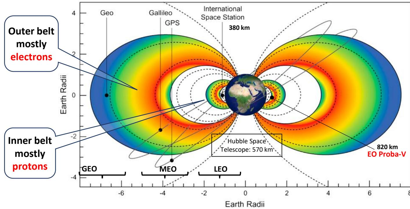
Different types of satellite orbits in relation to the Earth and the Earth's radiation belts. Most telecommunications satellites are in GEO, GNSS satellites such as Galileo and GPS are in MEO, and the international space station is in low Earth orbit (LEO). The slot region lies between the inner and outer radiation belts.
