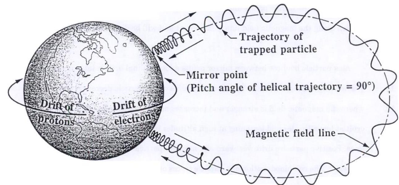
Motion of charged particles in the geomagnetic belts. A) gyration B) bouncing C) drift.
