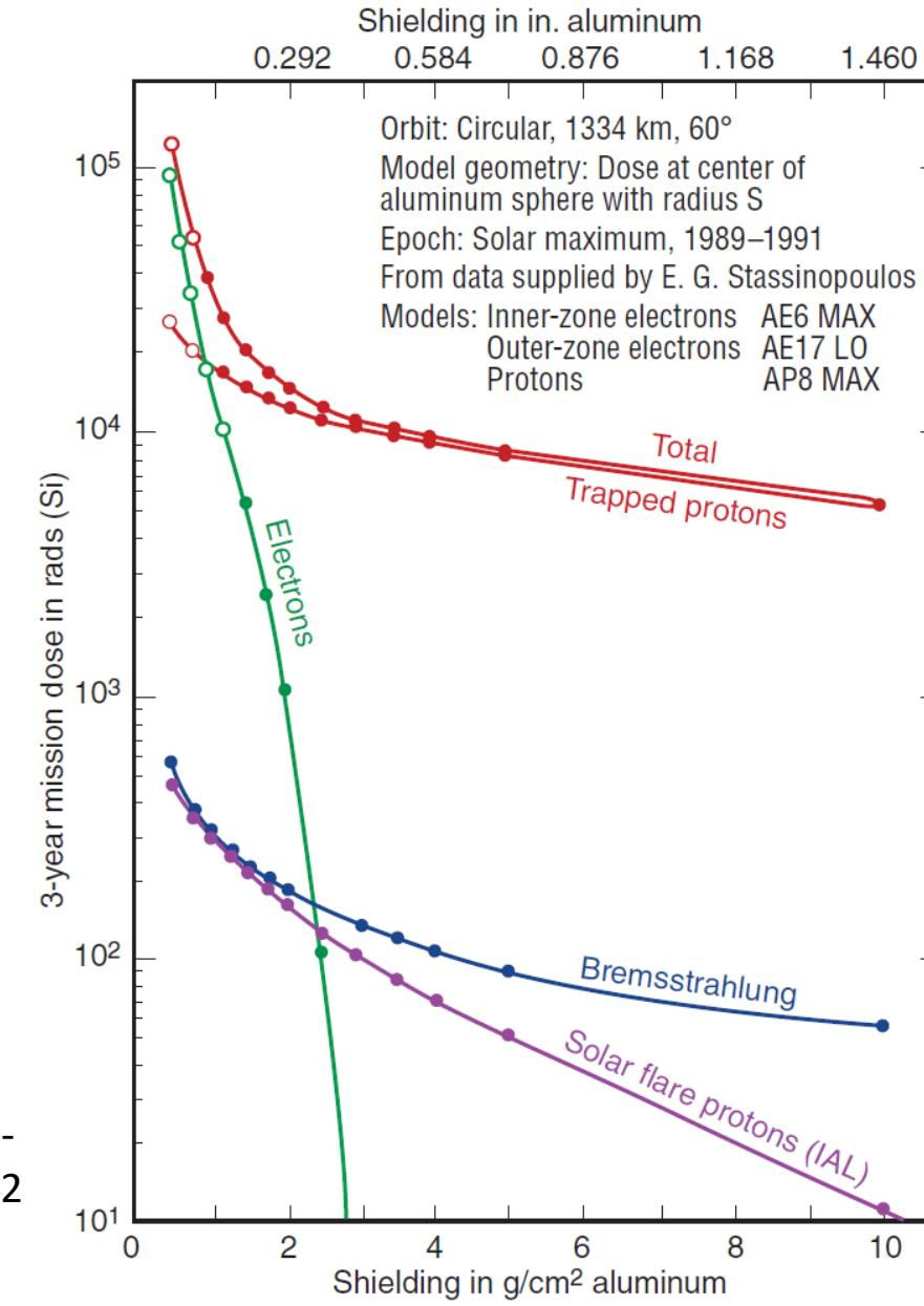
Dose-depth curve. The curve shows the effectiveness of shielding the electrons and the penetrating capability of the protons. The quasi-asymptotic total dose curve at the larger depths sets a floor of  $\sim 10,000$  rad (Si) below which it is impractical to shield.
