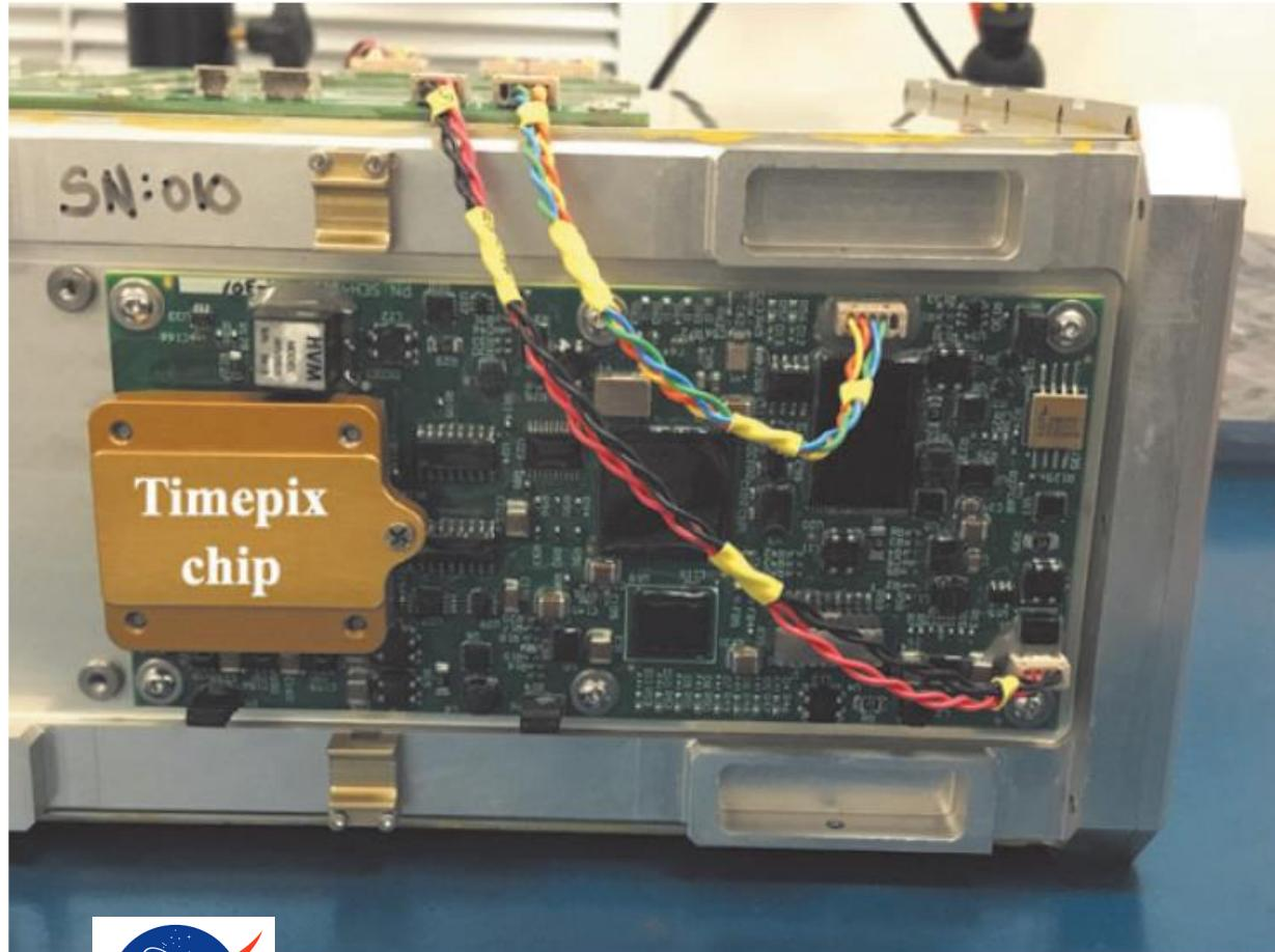
Readout electronics NASA-JSC, Radworks group
