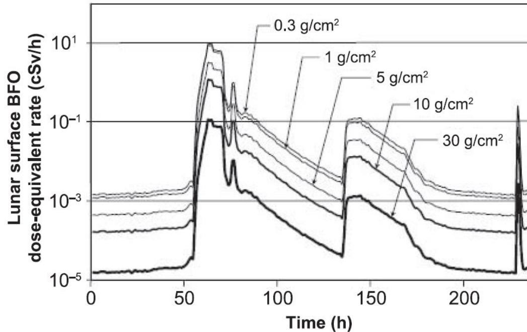
Lunar surface dose equivalent rate for blood-forming organs and effects of aluminum shielding for the large SPE on August 2, 1972. This event occurred between the Apollo 16 and 17 missions. Blood-forming organs dose equivalents are based on NCRP Report No. 132 recommendations. Note the high-dose-rate period of '20 h immediately after arrival of charged particles
