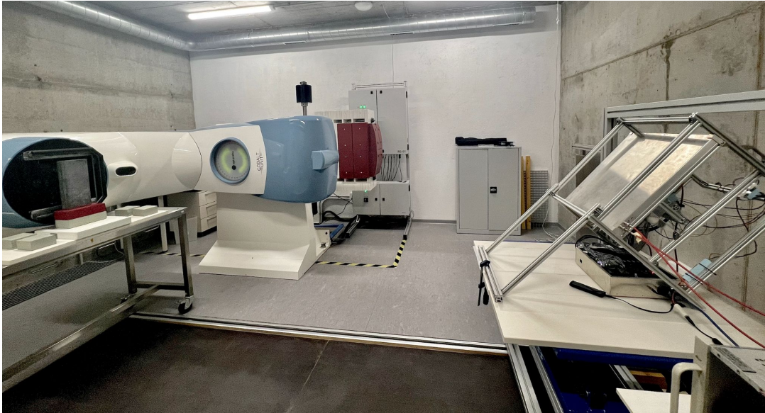
Fig. 9 - The detector under strong irradiation (Co-60) in Santiago's laboratory
