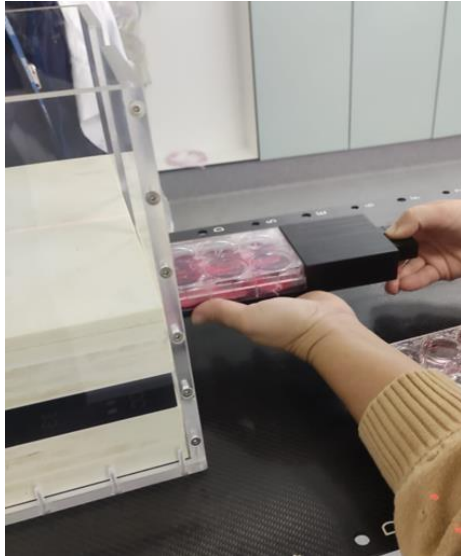
Positioning of the biological samples in the phantom for the irradiation with a clinical photon beam
