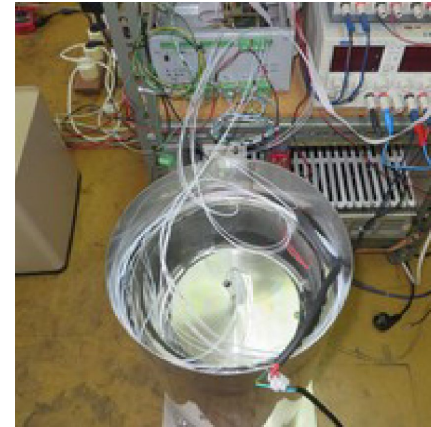
Home made oven with temperature sensors for control (MW).
