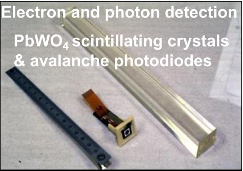
**Design Goal**: Measure the energies of photons from a decay of the Higgs boson **to precision of ≤ 0.5%**
