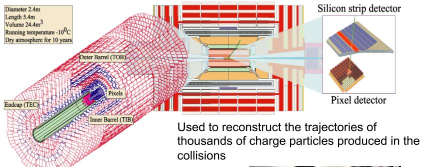
214m<sup>2</sup> silicon sensors 11.4 million silicon strips 65.9 million silicon pixels
