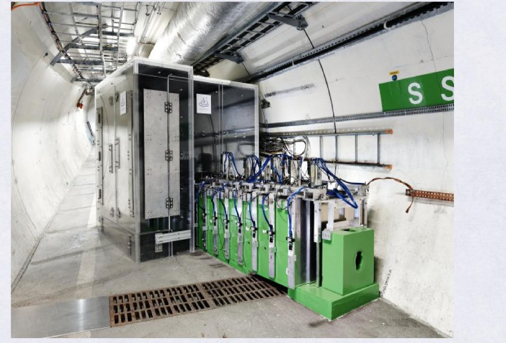
Current installation of the experiment at TI18, with the Cold Box/Neutron Shield surrounding the Veto System and Emulsion Targets
