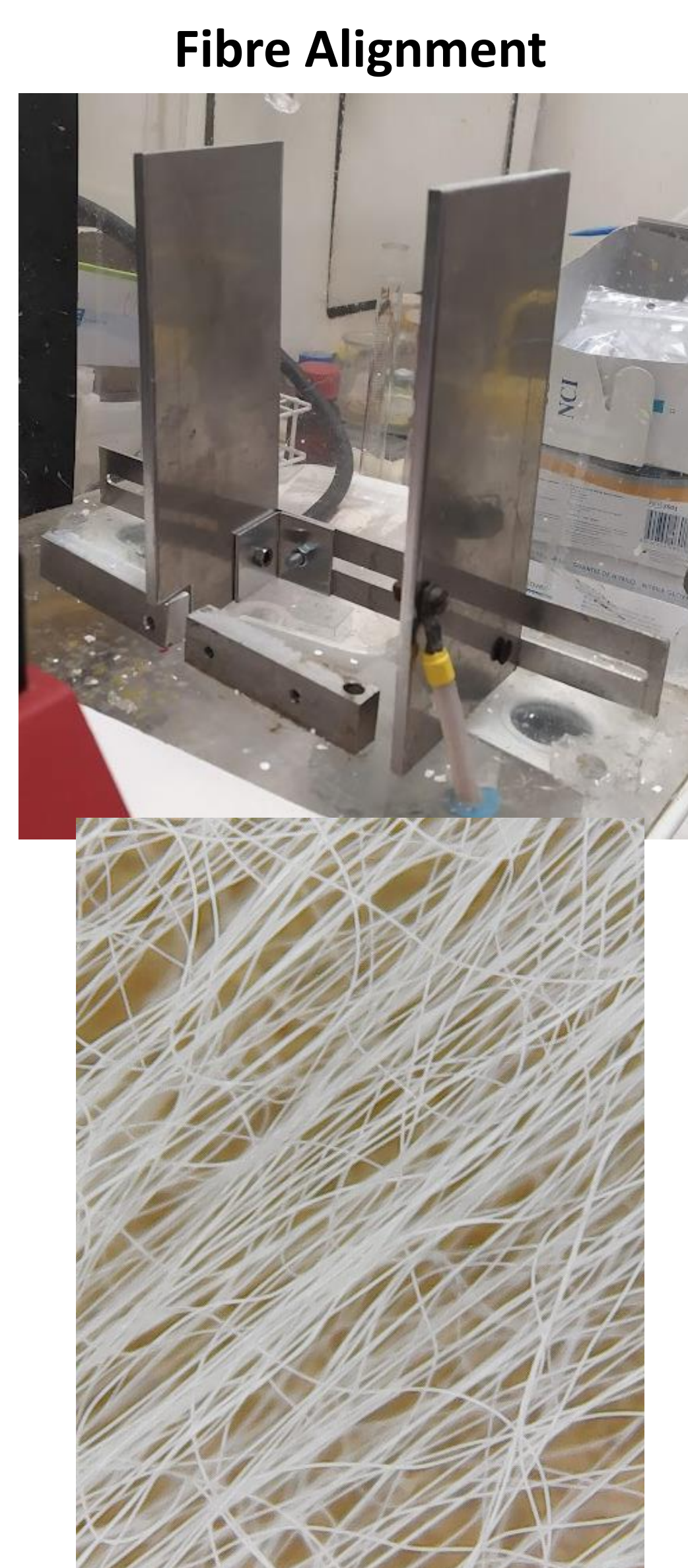
Figure 2. Collector used to obtain aligned electrospun fibres.
