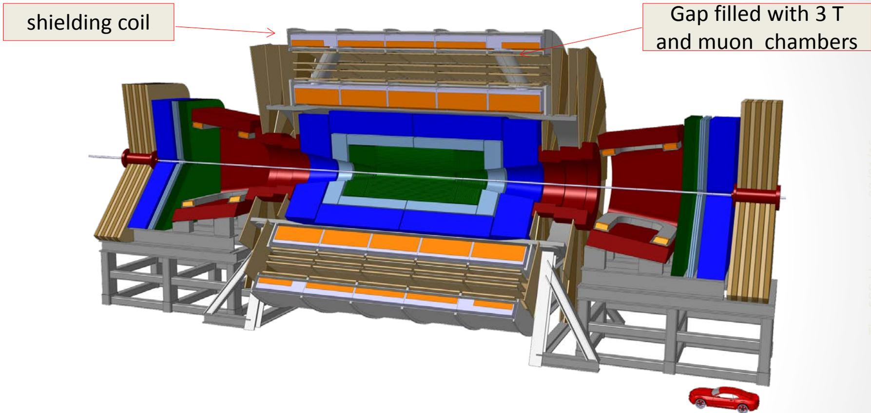
**Twin Solenoid:** 6 T, 12 m dia, 23 m long main solenoid + shielding coil
