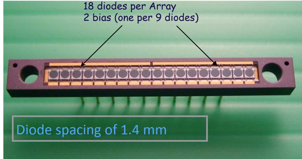
Si-PMTs insensitivity to B field and more granular readout should minimize space at outer radius for fibre bundles (if any) and electronics
