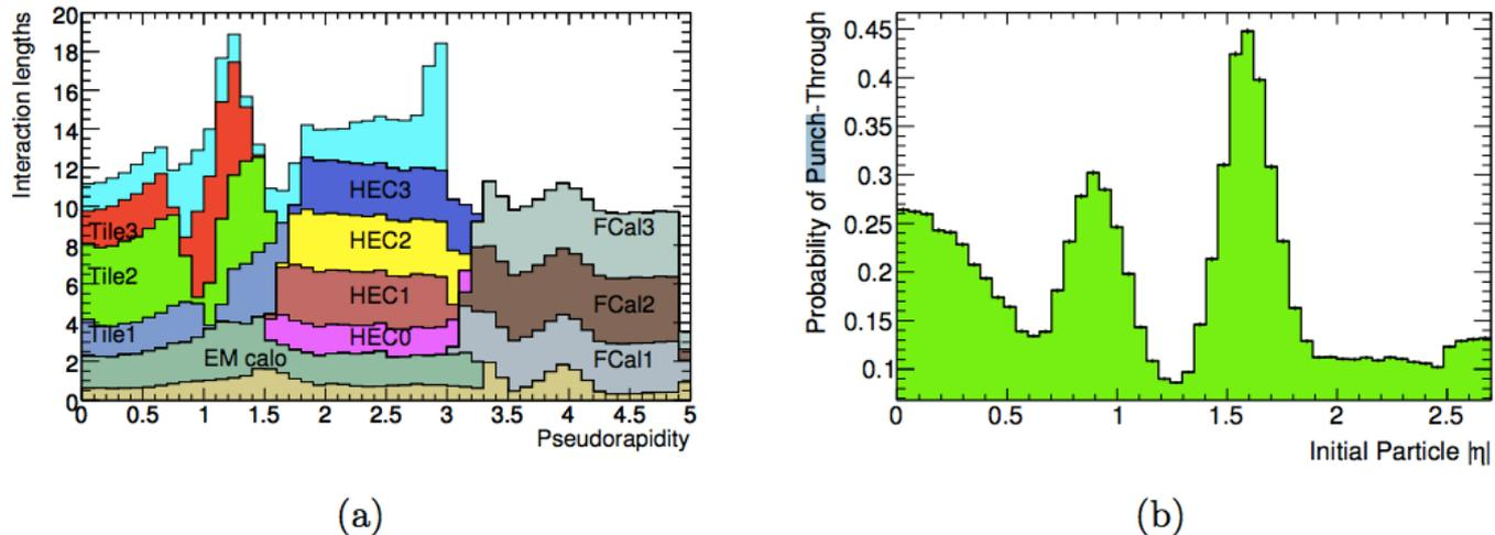
Figure 4.6: (a) Calorimeter material budget (in units of interaction length  $x_0$ ) versus pseudorapidity  $|\eta|$  [3]. (b) Probability to find one or more relevant punch-through particles in a single event vs. the initial particle's  $|\eta|$ .
