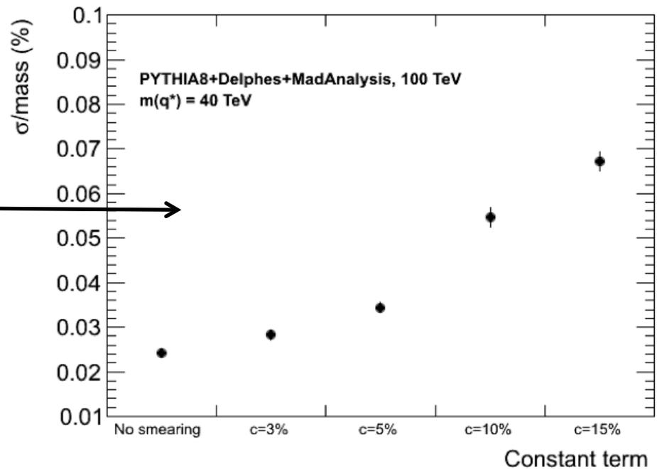
Longitudinal leakage increase hadron resolution constant term =>
