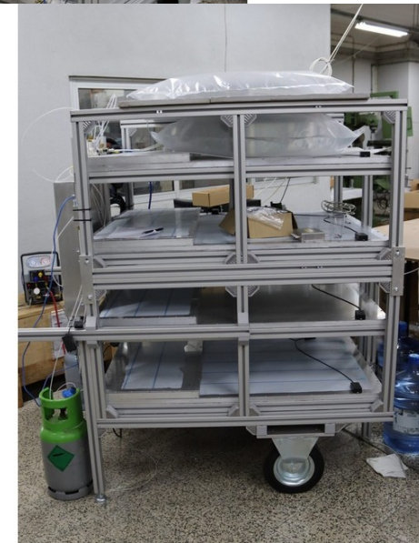
CorePix side view composed of 4 RPC detectors
