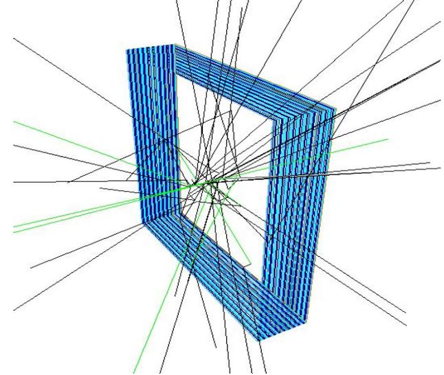
Simulation of 50 neutrons passing through the 10 Double-Gap RPC detector. Neutron tracks in green. Gamma-ray tracks in black.
