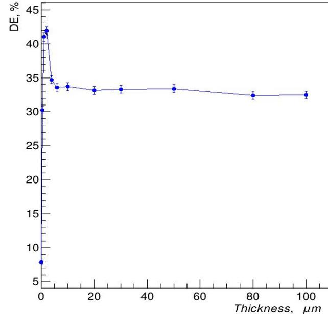
Detection Efficiency as a function of converter thickness. Orientation was maintained at 5°.
