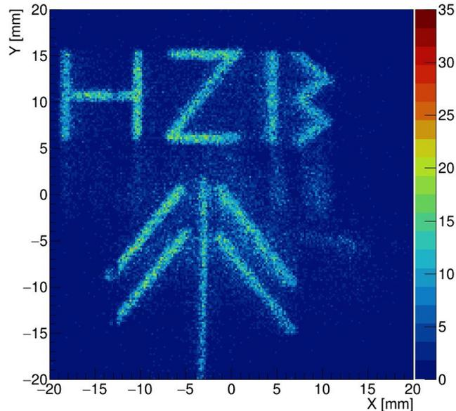
Reconstruction image obtained using a simplistic Centroid approach (200 x 200 bins)
