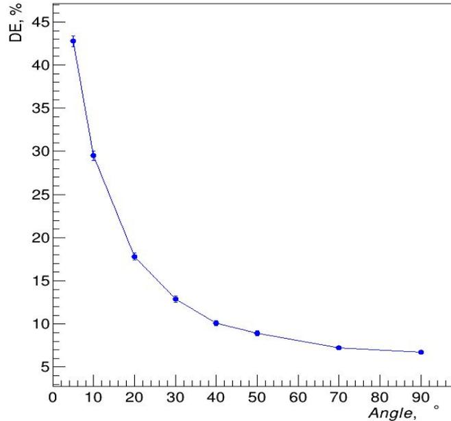
Detection Efficiency as a function of neutron beam angle of incidence. Zero degrees is the normal incidence. Converter thickness was maintained at 1.15  $\mu\text{m}$ .
