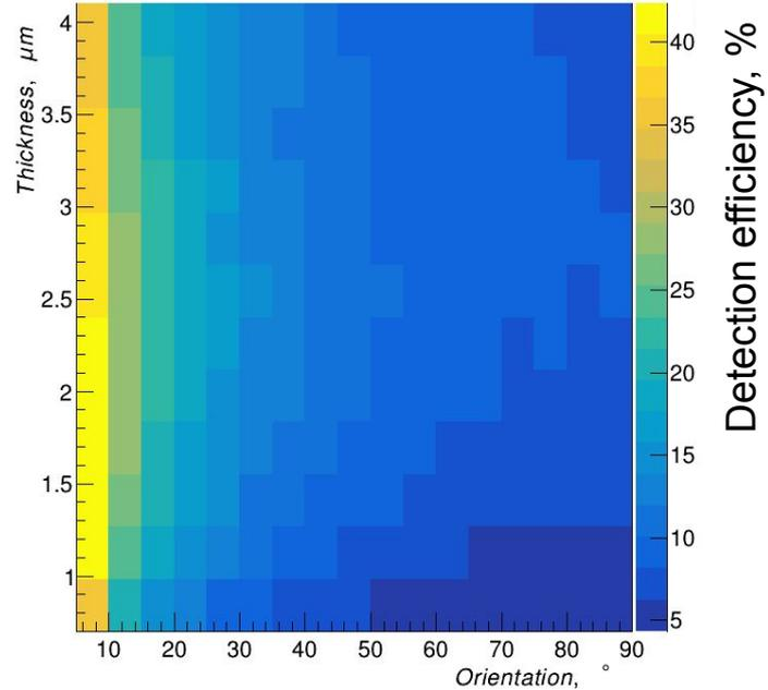
Detection efficiency as a function of the angle of incidence of neutrons and the converter thickness.
