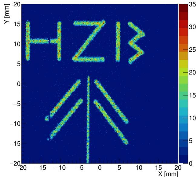
Reconstruction image obtained using an optimized Centroid approach ( $N = 4$ ; 200 x 200 bins)
