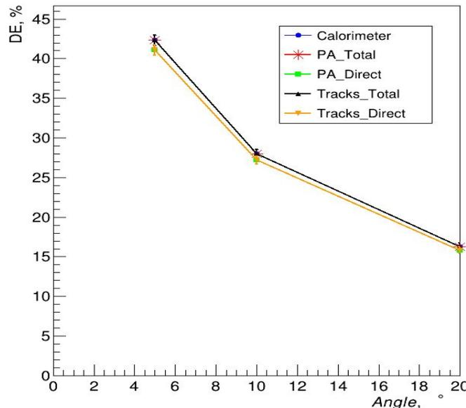
Detection efficiency as a function of neutron angle of incidence. **On the left:** Variation across all studied angles. **On the right:** Zoom in for angles between 0° and 20°.
