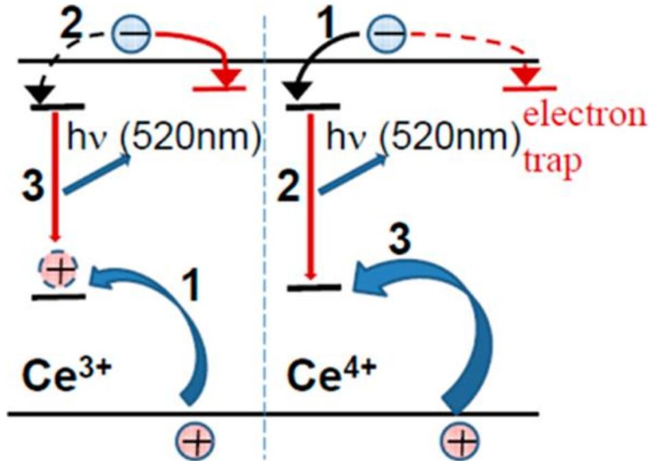
Presence of Mg<sup>2+</sup> increases number of Ce<sup>4+</sup> centers, compete with electron traps for electron capture in the initial instants of scintillator mechanism -> faster decay
