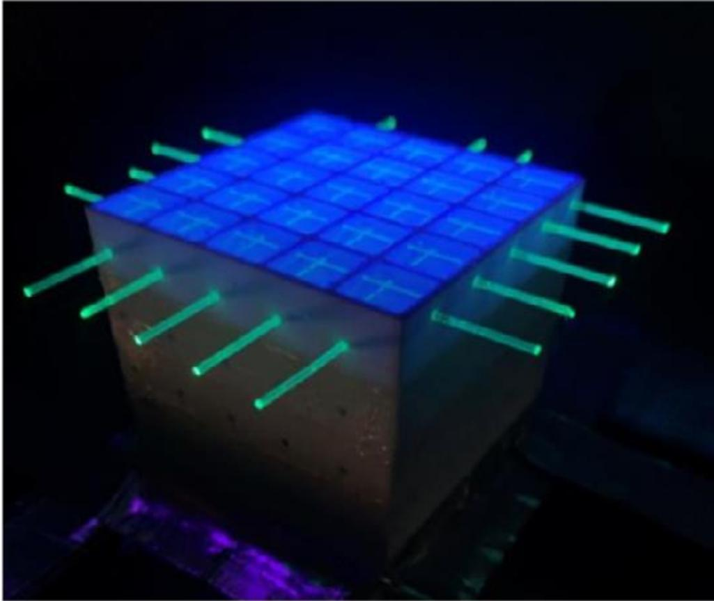
3D printed SuperCube, filled with WLS fibres (illuminated with UV light)
