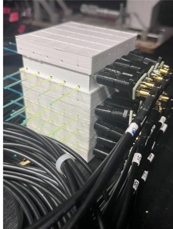
Detector ready for testing. Readout by SiPM.
