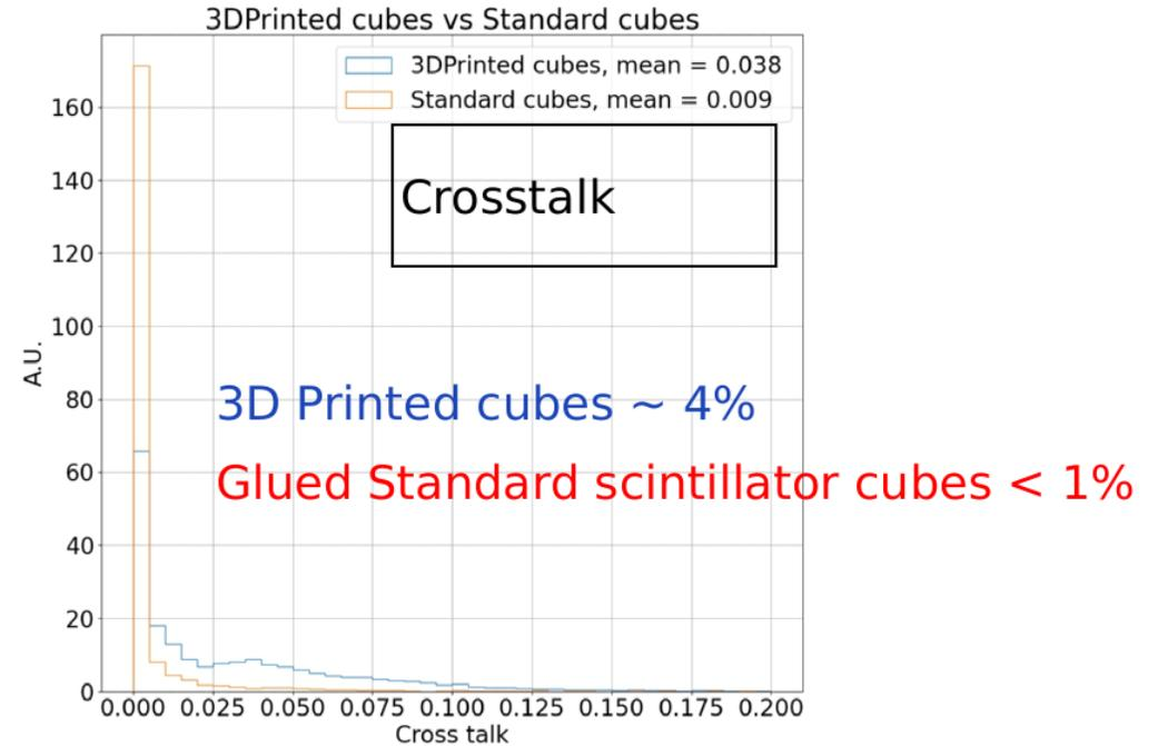
Successfully tested for the first time a totally 3D printed "final" plastic scintillator detector (no post-processing) with performance acceptable for a particle physics experiment
