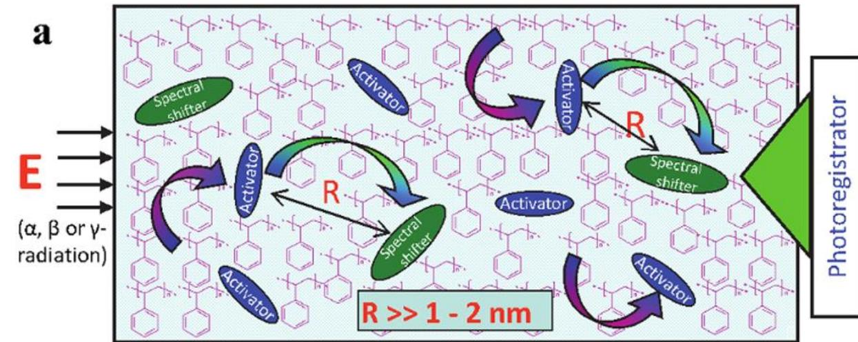
Typical organic scintillator, e.g., PS + pTp as activator and POPOP as spectral shifter to avoid light absorption by base and activator materials
