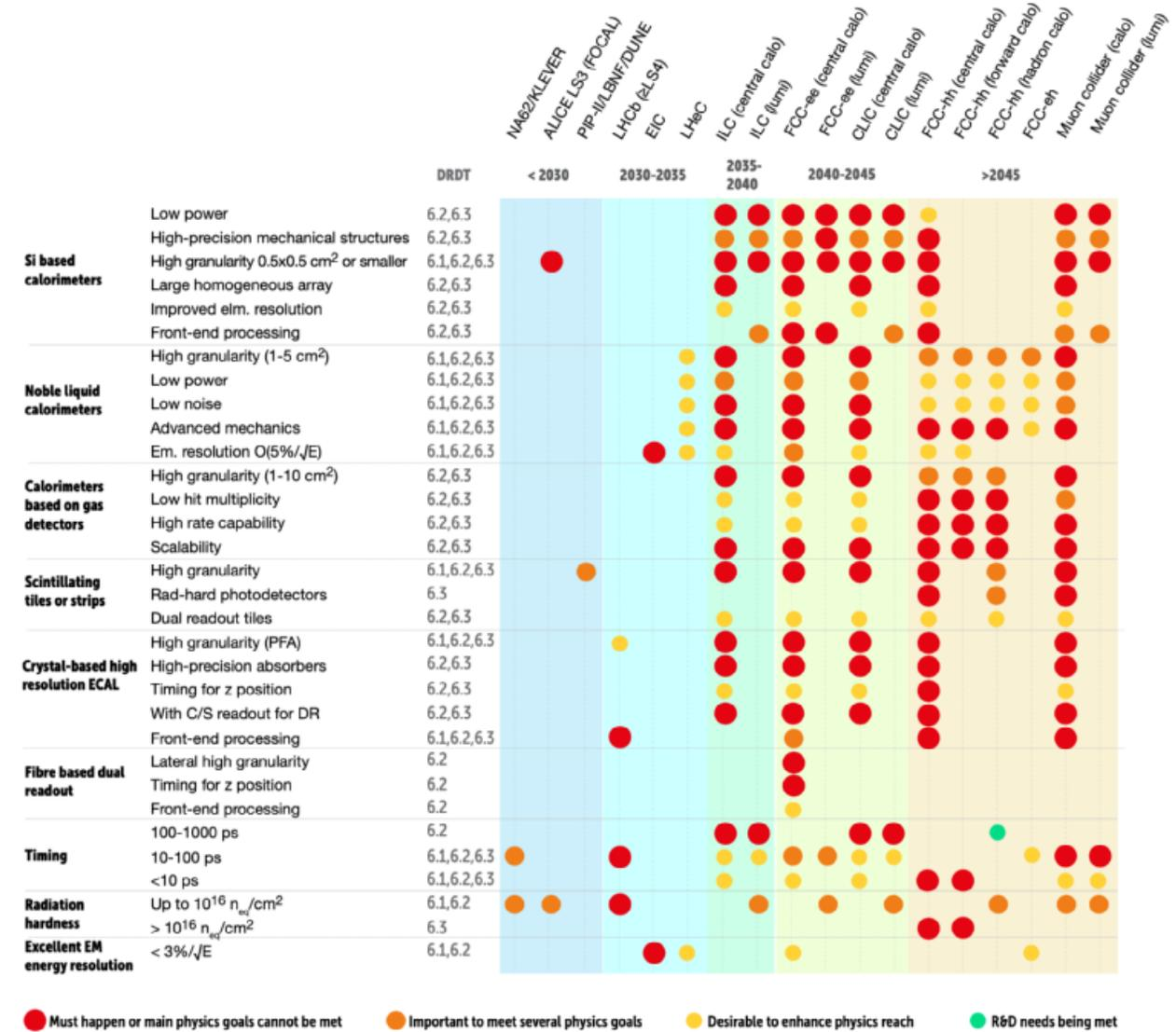
Technological needs for calorimetry
