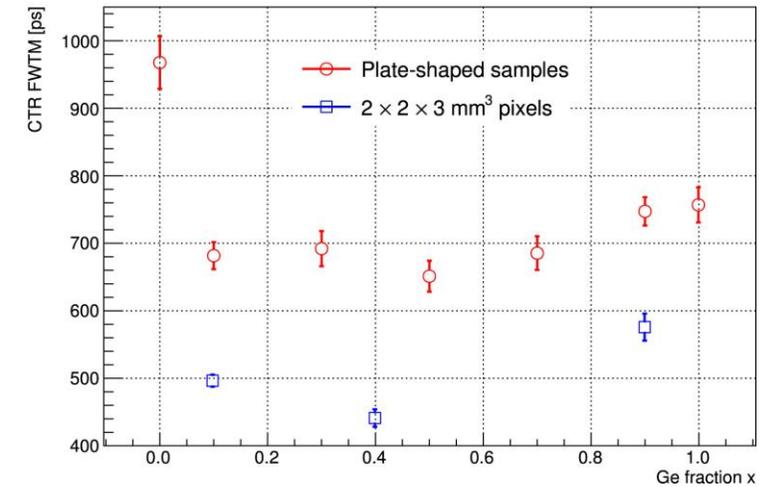
Coincidence time resolution @511Kev versus Ge fraction. It is optimal at 50% Ge fraction for plate shaped samples.
