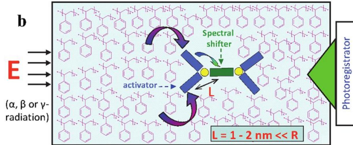
Engineer a spectral shifter that can be inserted in an activator molecule. Distance of order of nm ensures very good efficiency in the production of light by the spectral shifter for which the material is transparent
