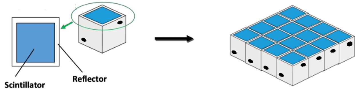
Simultaneous printing of scintillator and reflector with the holes in a single step is an efficient way of production
