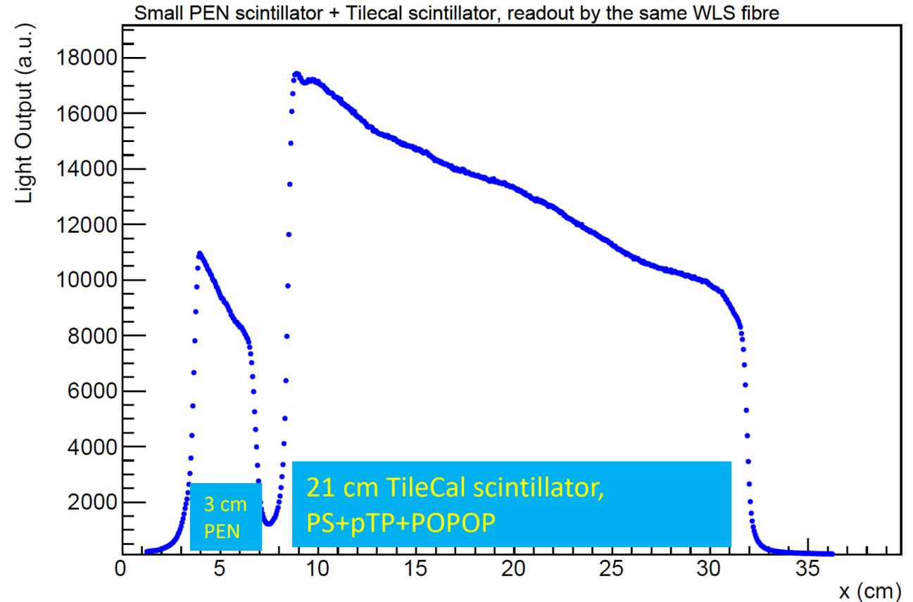
Scan using  $^{90}\text{Sr}$  source to excite the scintillators across the dashed line in the left figure.
