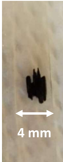
Crystals of Mn12 with the easy axis // to the external magnetic field
