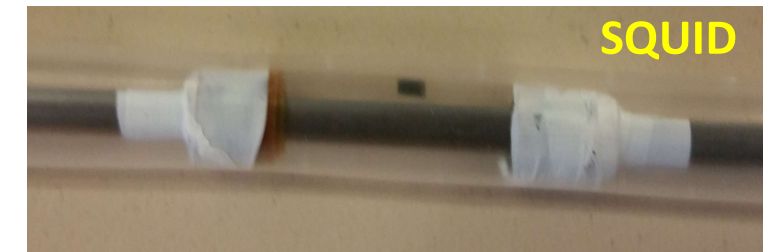
SQUID, NMR, EPR-II: semi-cylindrical geometry
