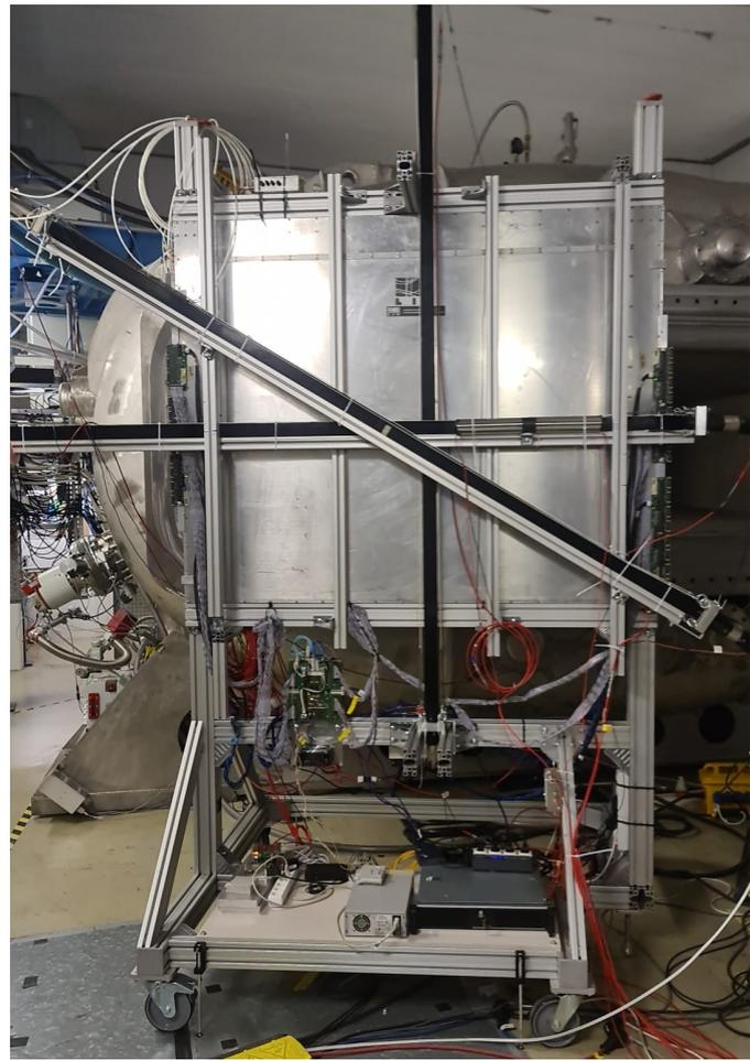
RPC @ R3B, GSI/FAIR, the crossing bars are Scintillators for calibration and efficiency
