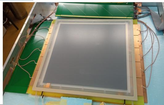
← 300x300 mm<sup>2</sup> prototype to be extended to 1 m<sup>2</sup>
