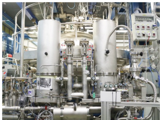
ARIA underground purification system for argon (DarkSide-20k)
