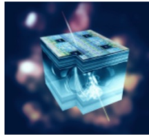
Illustration of microelectronics circuitry integrated with a detecting medium as a single monolithic active-state detector. (© ALICE collaboration)
