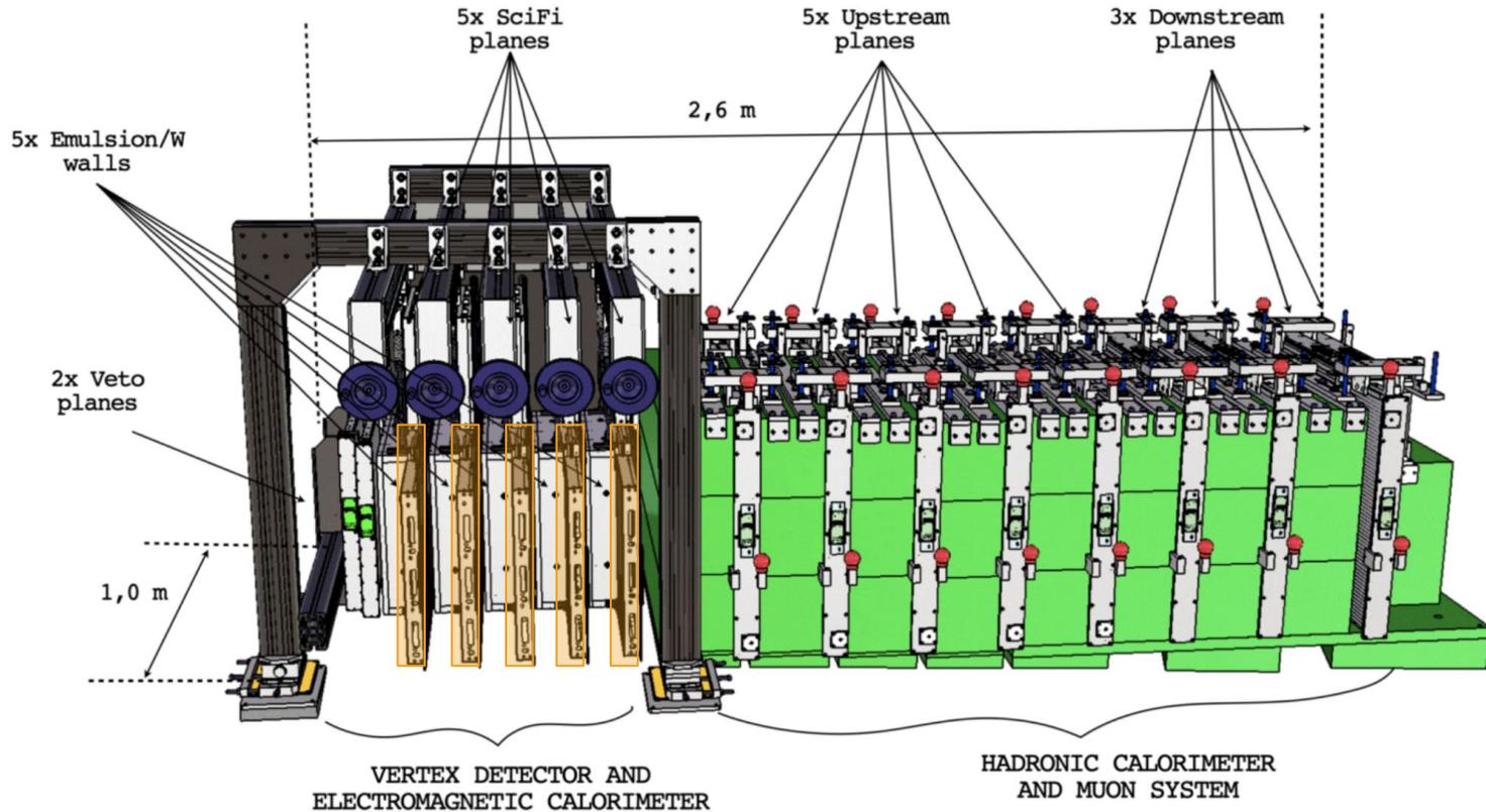
Each target wall is followed by a scintillating fibre detector station.
