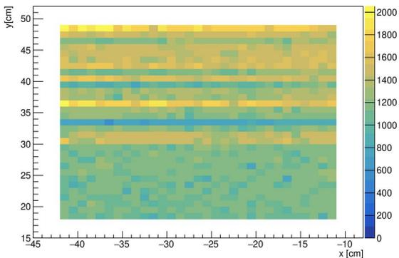
Measured muon track rate in Muon system ( $31 \times 31 \text{ cm}^2$ ):
