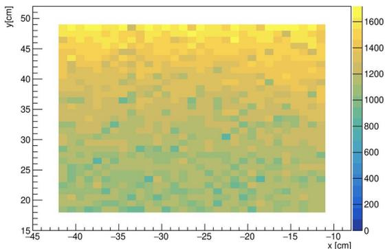
Measured muon track rate in SciFi ( $31 \times 31 \text{ cm}^2$ ):
