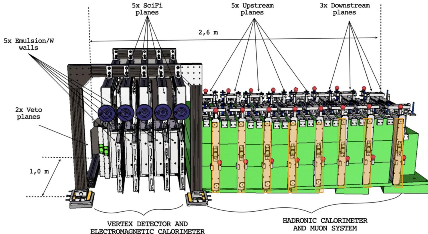
Fe-scintillator system with eight stations downstream of target.
