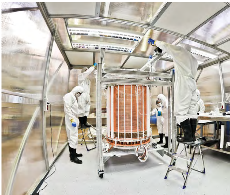
▲ FIG. 2: The heart of the XENON1T project, the Time Projection Chamber TPC after assembly in a clean room. @XENON1T team.
