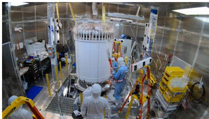
Time lapse of the LZ TPC being lowered into the ICV at the SAL clean room
