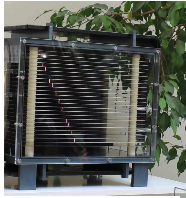
Track of a cosmic ray seen in a spark chamber at LIP
