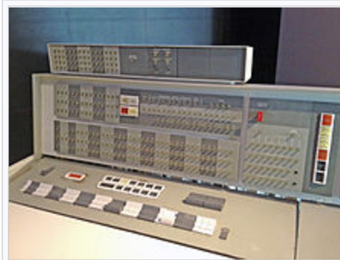
IBM 7094 operator's console showing additional index register displays in a distinctive extra box on top. Note "Multiple Tag Mode" light in the top center.
