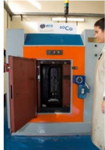
Fig. 7 – PRECISA22 – ^{60}\text{Co} irradiator used in the performed irradiations (Santos et al. s.d. )
