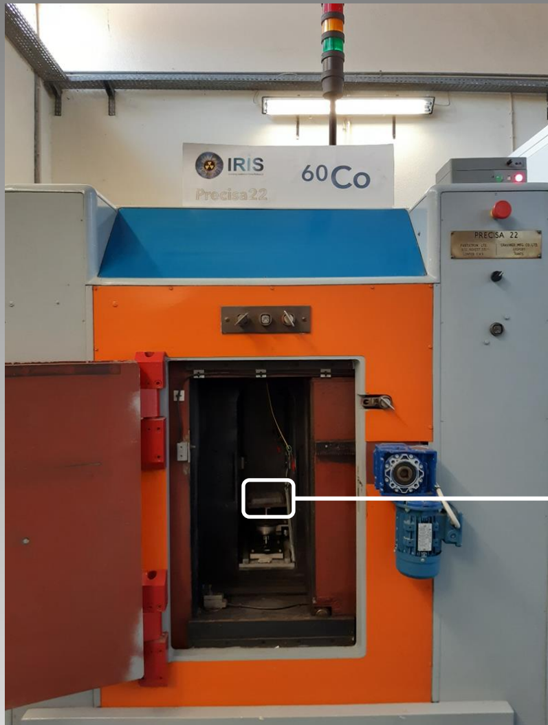
Fig. 03. a) Lead container where the sources, plates are located and where the irradiation takes place
