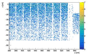
Most interaction vertices on Fe bars (less interactions on Scintillator Plates).
