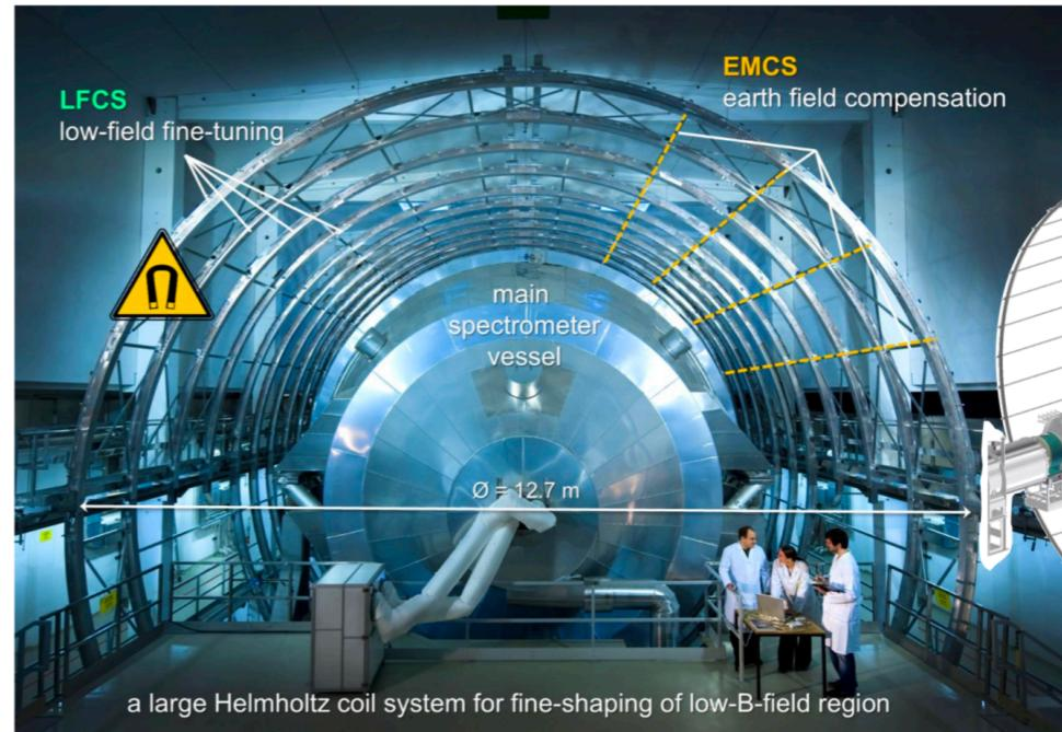
Outer air-coil system for B-field shaping:
