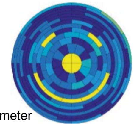
$e^-$  trajectories through different parts of the spectrometer have slightly different response functions
