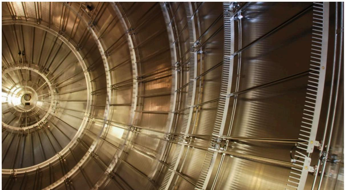
Inner electrode system for E-field shaping:
