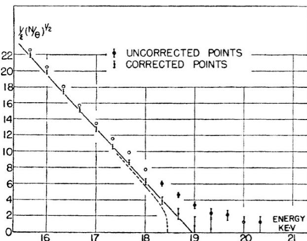
FIG. 2. "Kurie" plot of the end of the H<sub>3</sub> spectrum. The theoretical curve (shown dotted) corresponding to a finite neutrino mass of 500 ev (or 1 kev —see text) has been included for comparison.
