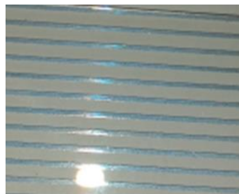
Strips (0.3 mm) on Al not well defined - More difficult to etch.
