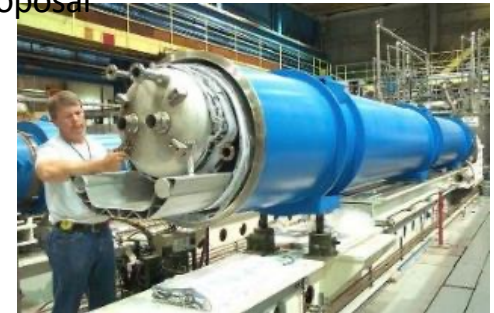
CERN LHC superconducting magnet
